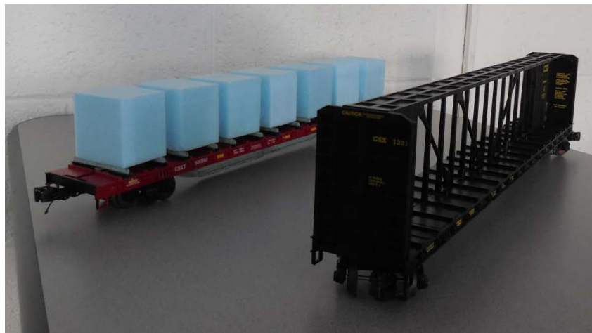
Figure 1. Model center beam car (right) and converted frac sand car with pods (left)
