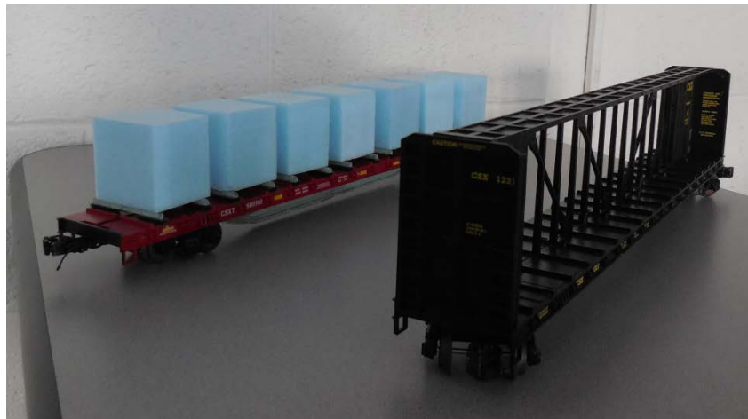
Figure 1. Model center beam car (right) and converted frac sand car with pods (left)
